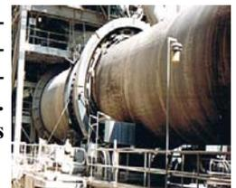
The bearings are inspected on an annual basis. They have seen an improved finish on the brass bearing surface and the shaft since they began using the new technology products. The thrust plates are cleaner and better polished, and the overall bearing condition has improved.
